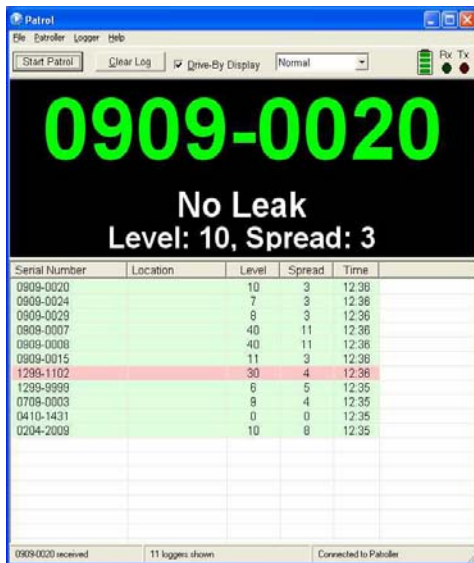
Standard Patrol Screen showing clear No Leak status
