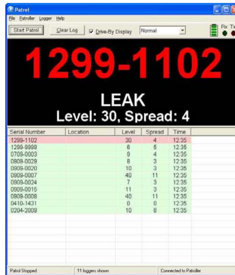
Standard Patrol Screen showing clear Leak status
